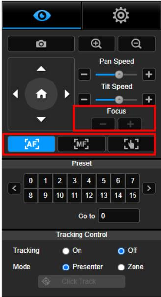
Switch to auto (AF) or manual (MF) focus. The manual focus use “+” and “-” to adjust focus. Select “+” to adjust focus to the far end and focusing on a far subject; select “-” to adjust focus to near end and focusing on a near subject.
