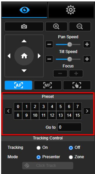
Select the number to view preset positions. User can also enter preset position number (0~255) in “Go to” column directly for a quickly calling section.
