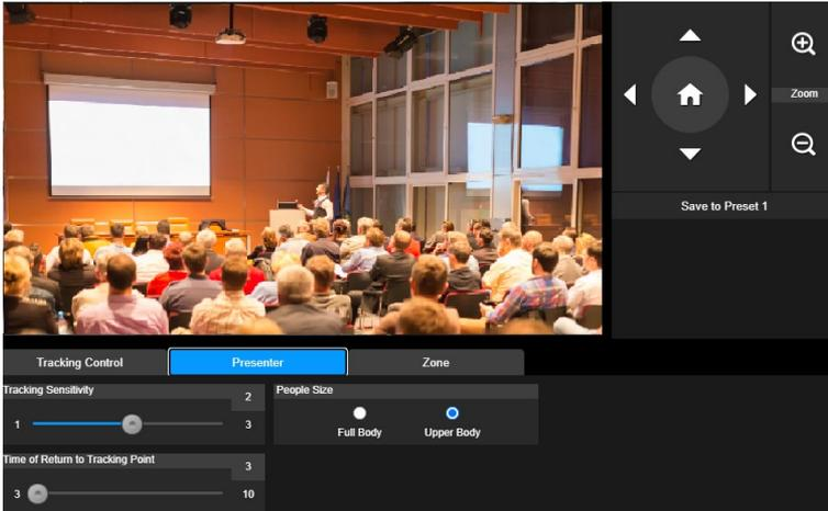
Camera will start tracking when object enters the tracking point.
