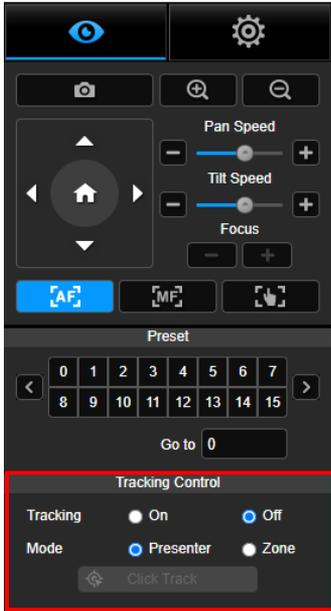
Enable/disable tracking function, select tracking mode, and operate one-click tracking function.
