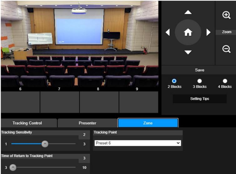
Set up 2 to 4 block areas for the camera. Each block is corresponding to one preset position. Camera will switch between preset positions when the presenter enters different blocks.
